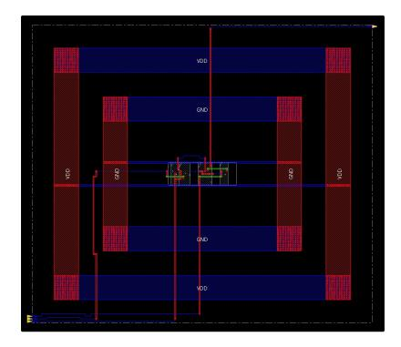
If you see white boxes and spacing errors when you route, your design is too constrained. Consider increasing the offset of your power rings by increments of 0.15.
