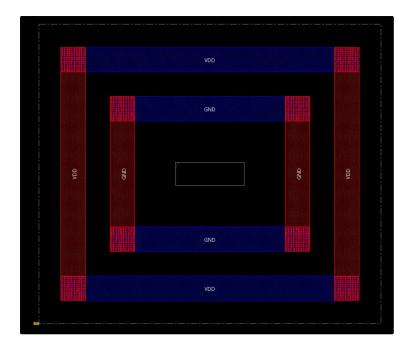
Connection to the global nets is done automatically if the nets are given the same names as was done in the setting of the power nets above. If all was done correctly, power planning should be finished.
