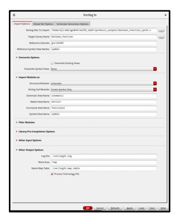
The import process should complete and may have a few errors or warnings. Ignore for now. Go to the schematic cell view created by the import process and open in Virtuoso. The synthesized optimized design should appear with the lowest level of hierarchy being the standard digital blocks
