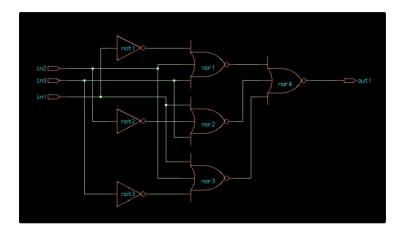
At this point, the RTL Compiler has generated an unoptimized version of the Verilog you provided. The final step is "synthesizing" the elaborated design, which optimizes the schematic already created and integrates your design with the gsc045\_svt standard cell library. While there are many optimization options available to you, we will skip them for this tutorial. The design can be synthesized with these following commands:
